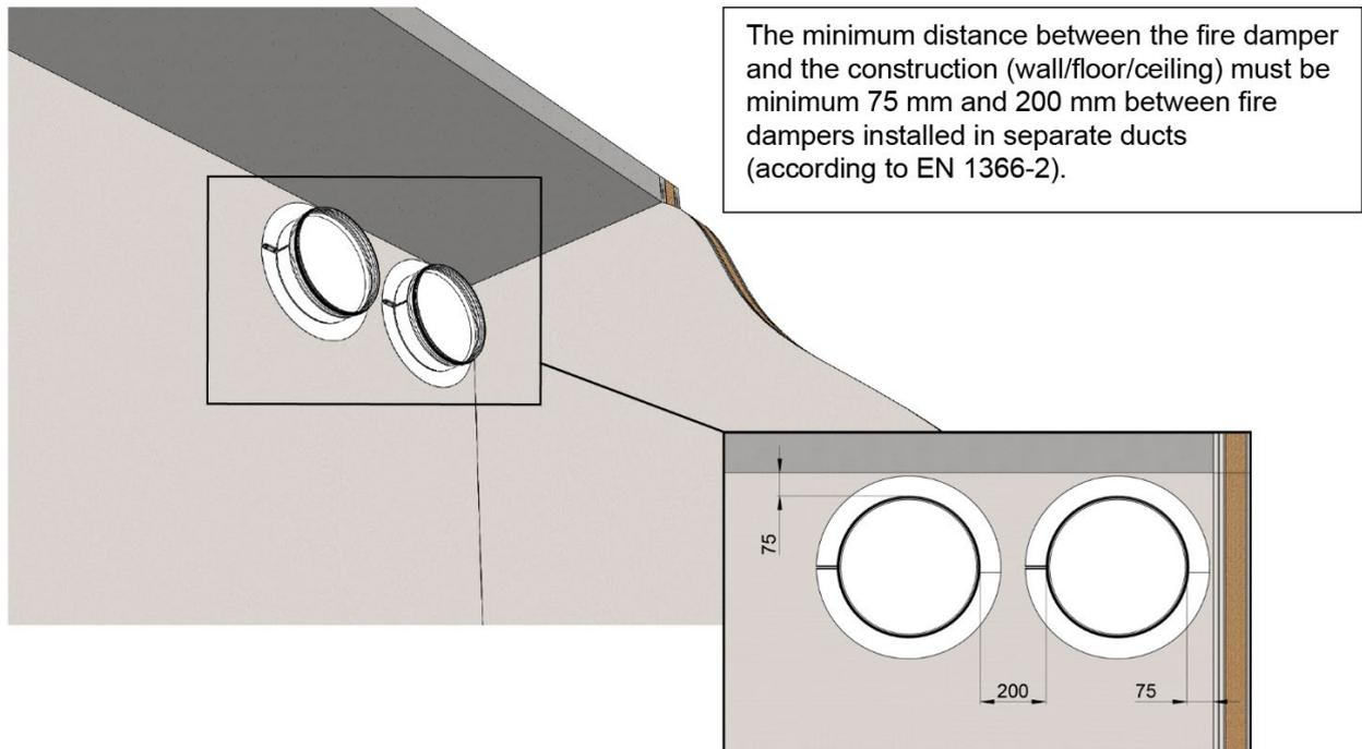
Fig. 3. The distance between the smoke control damper and construction
